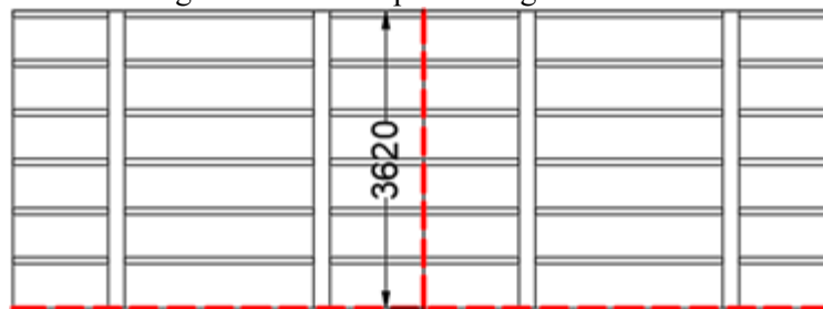
Figure 3. Welding Joints on Plates
