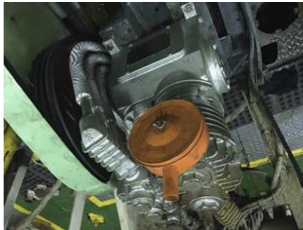
Figure 2. Two-level air compressor SV STELLA 28
